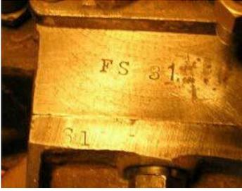
The engine number should be stamped and it might be on the clutch housing. It should look like the following and could start with F or FS.
